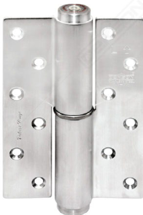
ESS HYD 6,2X4X3MM SSS Available Handing : Left or Right Capacity (max) : 60 KG / pair Material : SUS 304
