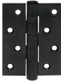
ESS DL 4X3X3MM 2BB MATT BLACK Capacity (max) : 75 KG / pair
