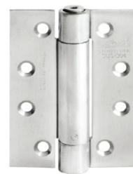
SPRING HINGE ESS SPR 4X3X3MM SSS Available : 4X4X3MM SSS Capacity (max) : 30 kg / pair Max Door Widht : 80 cm Material : SUS 304 (Not suitable to be applied to hotel lock doors)
